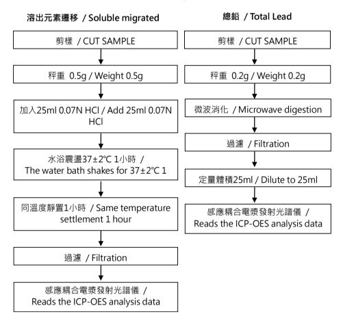
ASTM F963 分析流程圖 / Analytical flow chart- ASTM F963
